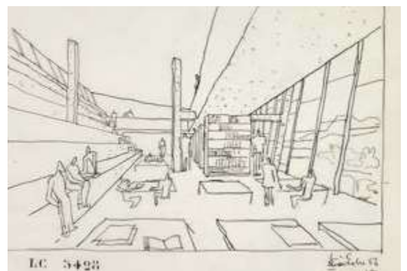
/ SKETCHES, 1956. ON THESE EARLY DRAWINGS, LE CORBUSIER STILL REPRESENTED LOAD-BEARING POLES. THE CREATION OF THE SELF-SUPPORTING ROOF ON CABLES MADE THEM UNNECESSARY.
